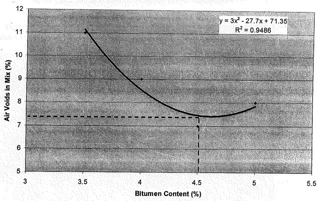
On the basis of above analysis the optimum bitumen content by percentage of the mix weight selected is 4.5 %. At the optimum binder content, the mix has achieved the maximum compacted density equal to 2.302 gms/cc. Similarly the air voids in the mix (by considering the bitumen absorption) has achieved a value of 7.5 %, which is acceptable as per the MS-2 recommendations.
